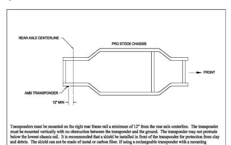
bracket, it is recommended that additional support like a tie wrap or similar be used. Do not rely solely on the cotter pin.
